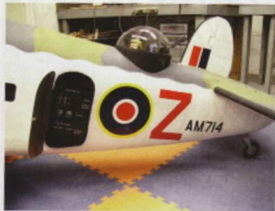
Radio switches are accessible through the entry hatch.
