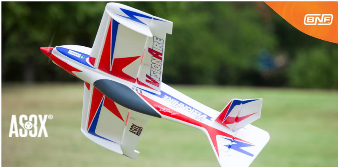
The Visionaire uses a 3s, 11.1v, 2200mah lipo for power. Motor and ESC are already installed. A Spektrum transmitter is required, as this is a BNF airplane.
